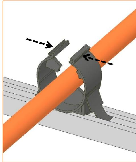
4. Slide elastomeric insulation over tubing ends and insert into Klo-Shure coupling pockets on both sides up to internal wall (MFG approved insulation adhesive on the ends of insulation is optional to further secure).
